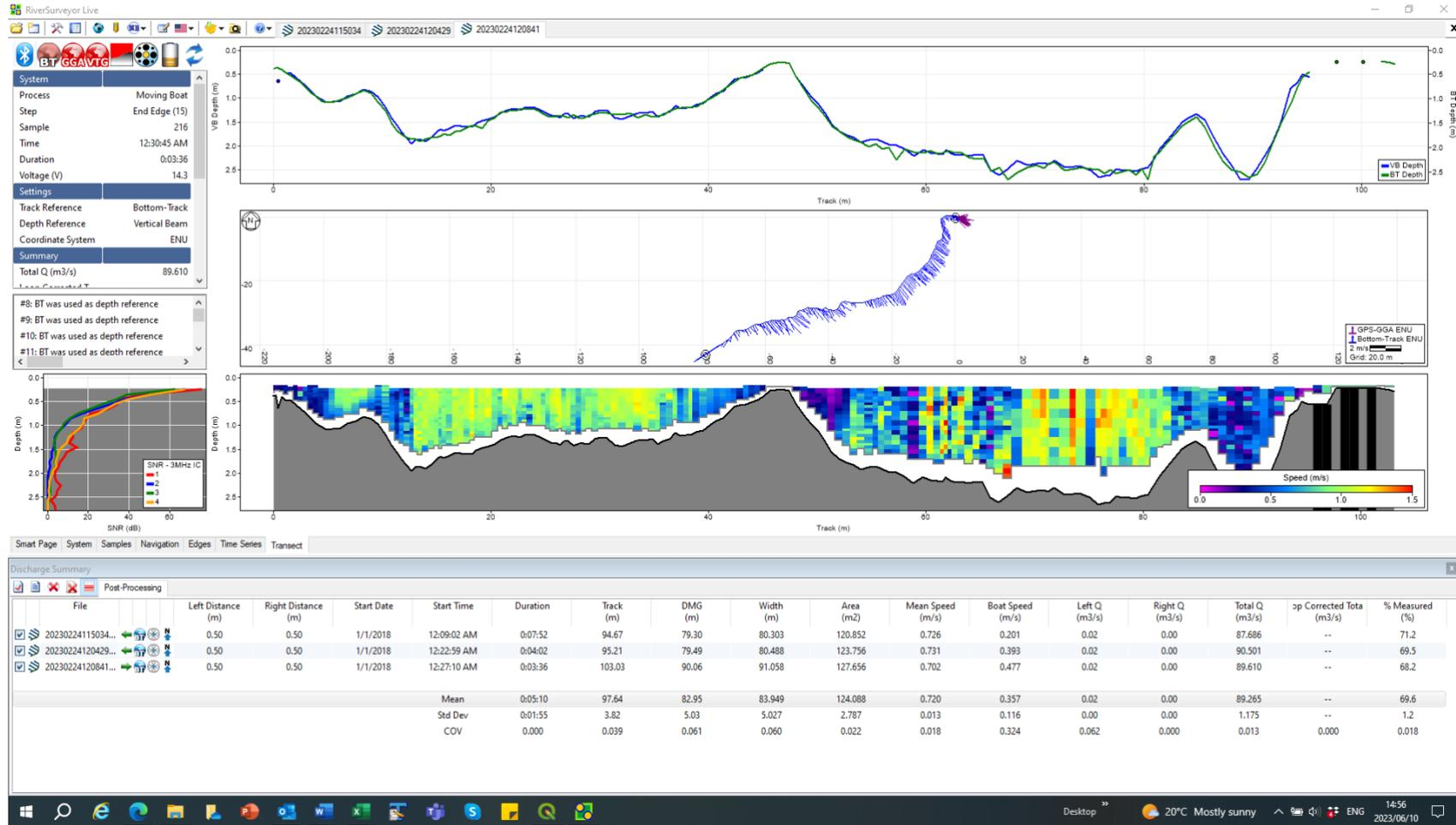
Appendix Figure 1: Sontek Acoustic Doppler Profiler discharge measurement along the Luvuvhu River at Pafuri Bridge on 24 February 2023 (89 m<sup>3</sup>/s)
