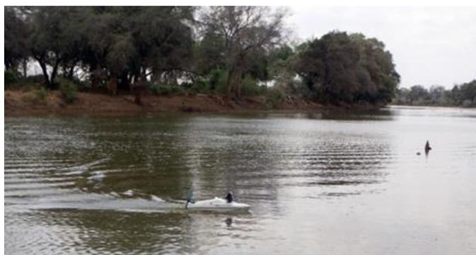
**Figure 4.16:** Survey equipment used for topographic and hydraulic data collection on the Luvuvhu River floodplain: left – surveying with a Trimble® Catalyst™ DA2 GNSS receiver; right – radio-controlled boat with onboard Lowrance HDS depth sounder on Nwambi Pan
