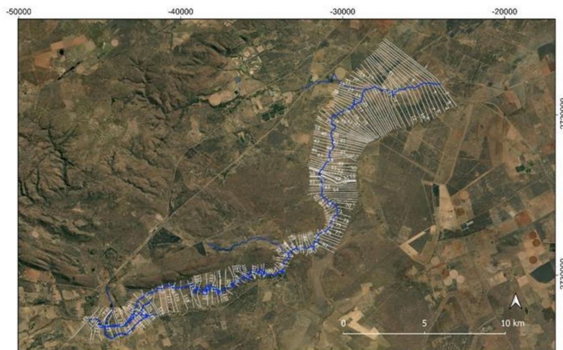
**Figure 4.5: 141 de-archived, reformatted and georeferenced cross-sections on the Nyl River floodplain, on a Bing satellite image; CRS is Hartebeeshoek94 Lo29**
