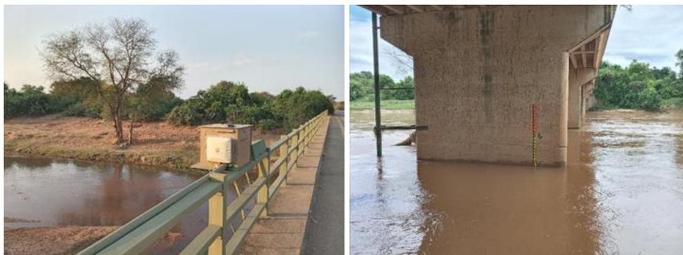
**Figure 4.13: DWS Station A9H032 on the Luvuvhu River at Pafuri Bridge - left: 21 October 2022; right: 24 February 2023, ~89 m<sup>3</sup>/s**
