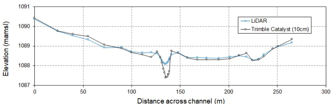
Figure 4.4: Cross-section derived from 2001 LiDAR data and the cross-section surveyed with a Trimble® Catalyst™ GNSS receiver (October 2022)
