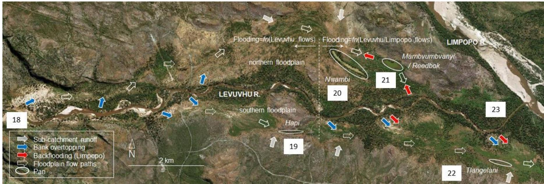
Figure 4.28: Water sources (viz. sub-catchment runoff, overtopping of the Luvuvhu River’s banks and backflooding from the Limpopo River) and flow paths across the Luvuvhu floodplain that result in filling of the pans; the EWR sites in DRIFT-Luvuvhu are numbered: 18\_Luvuvhu2, 19\_Hapi, 20\_Nwanbi, 21\_Mambvumbvanyi, 22\_Tlangelani, 23\_Luvuvhu3
