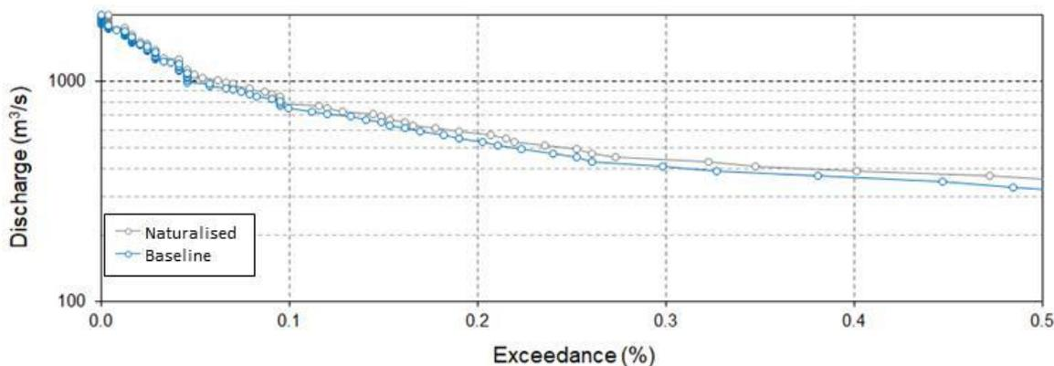
**Figure 4.43: Modelled (high flow) discharge-exceedance plot for the lower Luvuvhu River (KNP) for Naturalised and PES flow scenarios**
