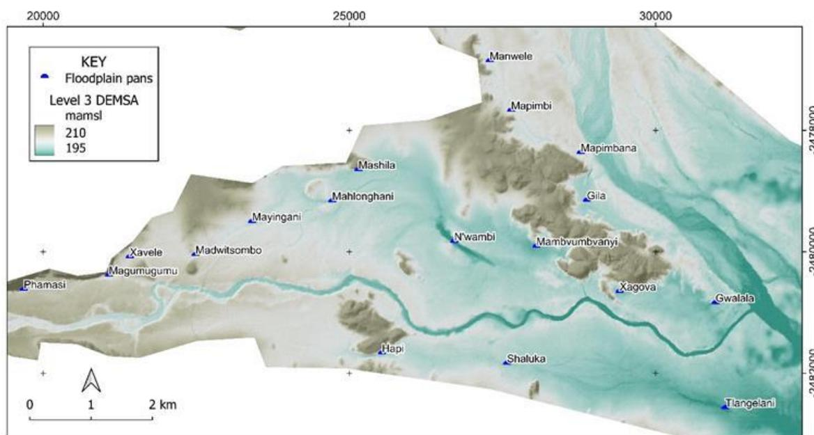
**Figure 4.12: Digital Elevation Model of the Luvuvhu River floodplain to the Limpopo River confluence (~0.5 km east of the Gwalala Pan) from the 2 m resolution Level 3 DEMSA2 DTM; CRS is Hartebeeshoek94 Lo31**
