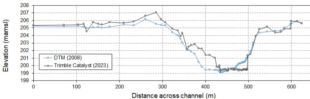
Figure 4.17: Cross-section surveyed across the Luvuvhu River; differences between profiles do not necessarily reflect survey errors, but also geomorphological change (2008 to 2023) that is evident from the underlying aerial photography
