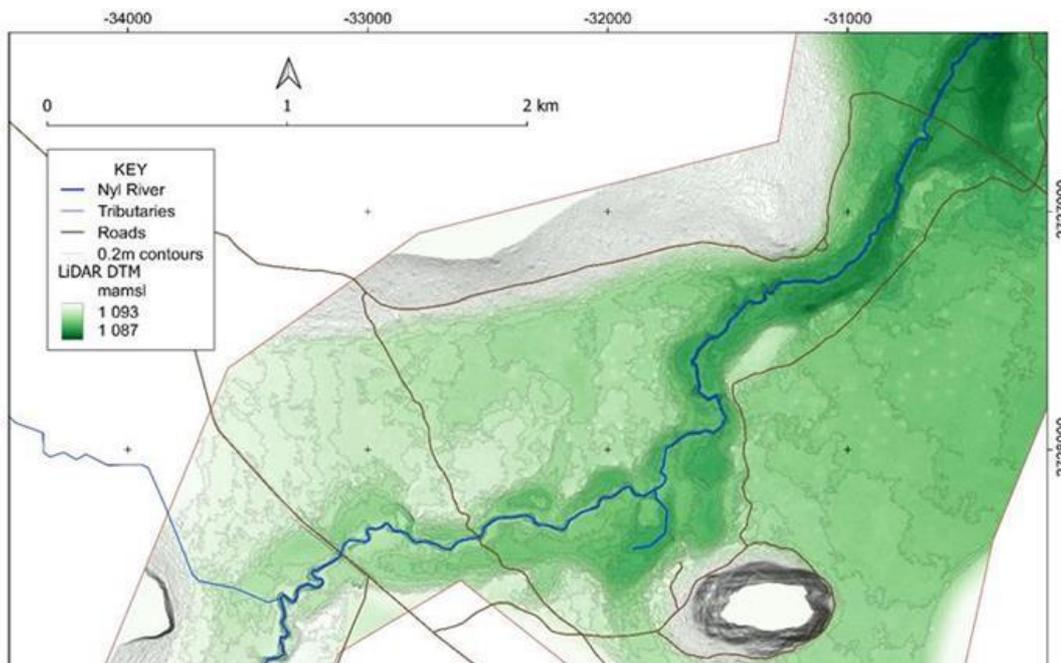
Figure 4.3: DTM and superimposed 0.2 m contours at Nylsvley; CRS is Hartebeeshoek94 Lo29
