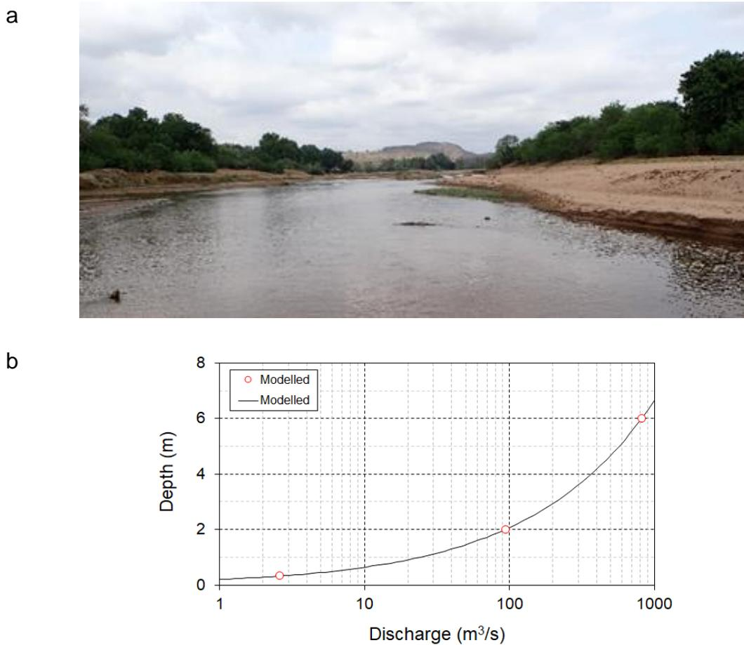
Figure 4.34: a) Photograph of the sand-bed river at a site on the lower Luvuvhu ~900m upstream of Pafuri Bridge (photograph J. Makenzie); b) modelled rating relationship
